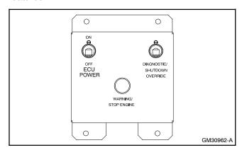
Figure 3-24 John Deere Engine Control Box
